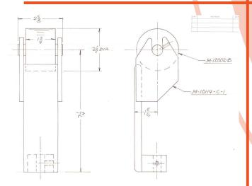
TYPE 4. (M10504-C-1) Top Bearing Assembly. General purpose work where heavier grinding is needed. Features heavier construction, increased width and rubber covered contact wheel. Permits working on wheel, platen or slack of belt. Will fit internal opening 2-3/4" square. Accommodates abrasive belts 2" x 90".
