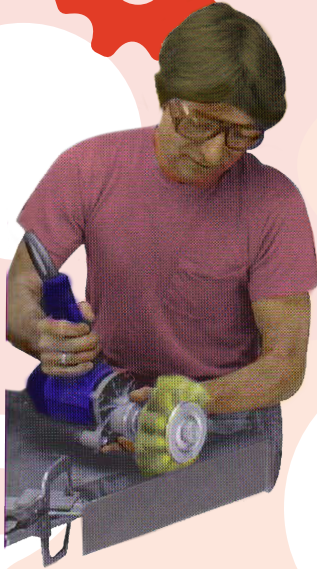
Blending operation on fabricated stainless part
